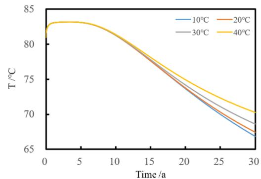
**Figure 4. Production temperature under different injection temperature conditions**
