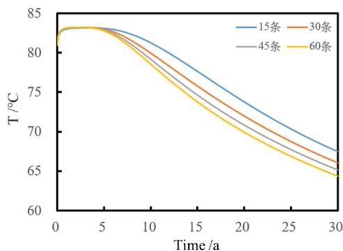
Figure 6. Production temperature under different fracture number conditions
