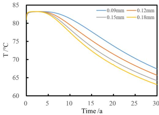
Figure 5. Production temperature under different crack opening conditions
