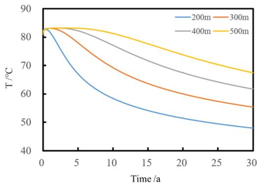
**Figure 2. Production temperature of different well spacing**
