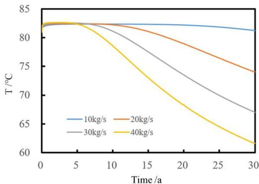
**Figure 3. Production temperature at different water injection rates**
